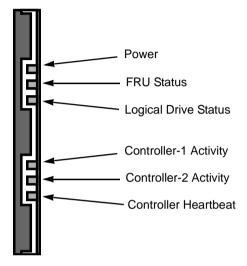
When boot-up is finished and the VTrak is functioning normally:
